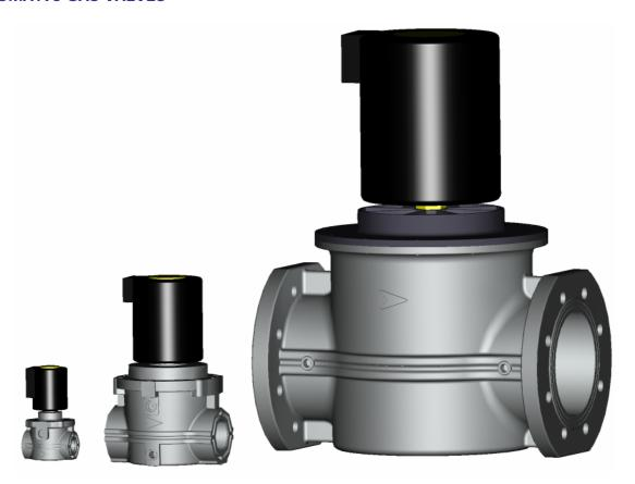
Gas Solenoid Valves are used for safety and control of gas for shut-of in gas feed pipes. Suitable for various gases, including Natural gas, Propane and LPG  $\frac{1}{4}$ " Inlet and outlet plugs suitable for CPI switch, pressure gauge, connection to proving and interlock Systems
